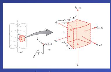
$$\frac{1}{r}\frac{\partial}{\partial r}\left(kr\frac{\partial T}{\partial r}\right) + \frac{1}{r^2}\frac{\partial}{\partial \phi}\left(k\frac{\partial T}{\partial \phi}\right) + \frac{\partial}{\partial z}\left(k\frac{\partial T}{\partial z}\right) + \dot{q} = \rho c_p \frac{\partial T}{\partial t}$$
