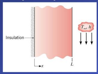
KNOWN: Plane wall, initially at a uniform temperature, is suddenly exposed to convective heating.
