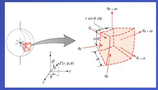
$$\frac{1}{r^2} \frac{\partial}{\partial r} \left( kr^2 \frac{\partial T}{\partial r} \right) + \frac{1}{r^2 \sin^2 \theta} \frac{\partial}{\partial \phi} \left( k \frac{\partial T}{\partial \phi} \right) + \frac{1}{r^2 \sin \theta} \frac{\partial}{\partial \theta} \left( k \sin \theta \frac{\partial T}{\partial \theta} \right) + \dot{q} = \rho c_p \frac{\partial T}{\partial t}$$
