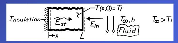
**ASSUMPTIONS:** (1) One-dimensional conduction, (2) Constant properties, (3) No internal heat generation.
