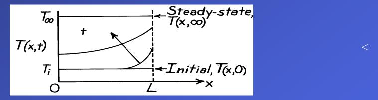
Note that the gradient at x = 0 is always zero, since this boundary is adiabatic. Note also that the gradient at x = L decreases with time.
