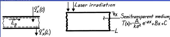
**ASSUMPTIONS:** (1) Steady-state conditions, (2) One-dimensional conduction in medium, (3) Constant properties, (4) All laser irradiation is absorbed and can be characterized by an internal volumetric heat generation term  $\dot{q}(x)$ .
