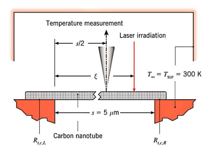
Determine the two contact resistances,  $R_{t,c,L}$  and  $R_{t,c,R}$  at the left and right ends of the nanotube, respectively. The experiment is performed in a vacuum with  $T_{\rm sur} = 300$  K. The nanotube thermal conductivity and diameter are  $k_{\rm cn} = 3100$  W/m·K and D = 14 nm, respectively.
