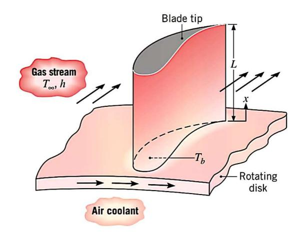
The blades, which are fabricated from Inconel,  $k \approx 20 \text{ W/m} \cdot \text{K}$ , have a length of L = 50 mm. The blade profile has a uniform cross-sectional area of  $A_c = 6 \times 10^{-4} \text{ m}^2$  and a perimeter of P = 110 mm. A proposed blade-cooling scheme, which involves routing air through the supporting disc, is able to maintain the base of each blade at a temperature of  $T_b = 300^{\circ}\text{C}$ .
