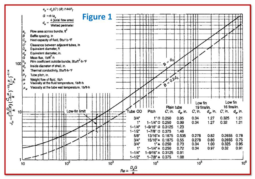
Correlation for shell-side heat-transfer coefficient. For rotated square tube layouts, use the parameter values for square pitch and replace  $P_T$  with  $P_T/\sqrt{2}$  in the equation for  $a_s$
