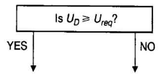
Exchanger is thermally suitable
