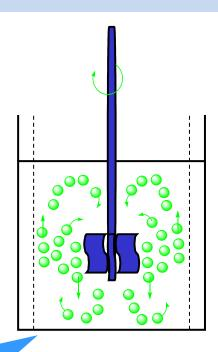
Suspension polymerization in polymer micro-droplets
