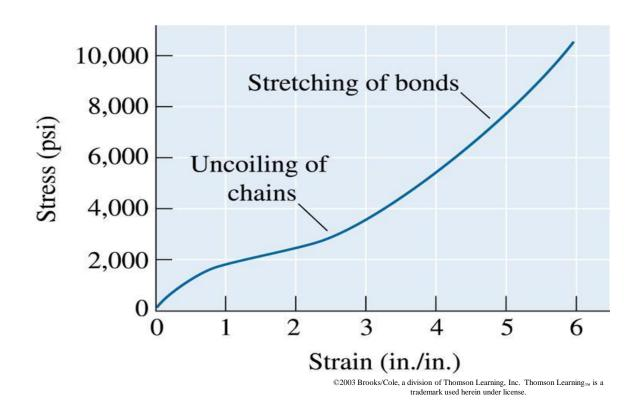
The stress-strain curve for an elastomer. Virtually all of the deformation is elastic; therefore, the modulus of elasticity varies as the strain changes.
