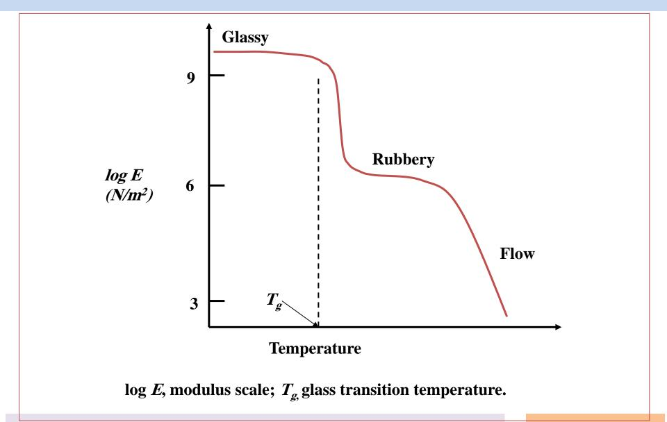
Effect of temperature on tensile modulus (log E scale) of various polymers
