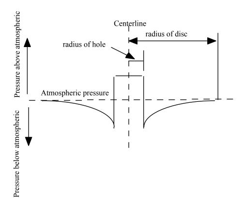
$Q = \frac{1 \text{ L}}{2 \text{ s}} = 0.5 \frac{\text{L}}{\text{s}}$  The area of the periphery is 5.57  $A = \pi Dh = \pi \cdot 35 \text{ mm} \cdot 0.2 \text{ mm} = 22.0 \text{ mm}^2$ , so the velocity at the perimeter is  $V = \frac{Q}{A} = \frac{0.5 \frac{L}{s}}{22 \text{ mm}^2} \cdot \frac{10^6 \text{ mm}^3}{L} = 22.736 \frac{\text{mm}}{s} = 22.7 \frac{\text{m}}{s}$
