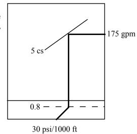
(b) To do it using Fig 6.10 one sees that it is the same type of problem as Ex. 6.5, the Type 2 problem in Table 6.3, which leads to a trial-and error solution. This is very similar to that shown in Table 6.5, and is shown below
