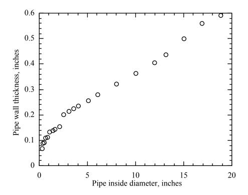
However if one fits the sizes from 1/8 to 2 inches nominal, one finds  $t = 0.0719 \, \text{in} + 0.0454 \, D_{\text{inside}}$ ,  $R^2 = 0.897$ . One can get  $R^2 = 0.976$  by fitting a quadratic to this data set, showing that the values for the smaller pipes do not correspond very well to this equation.
