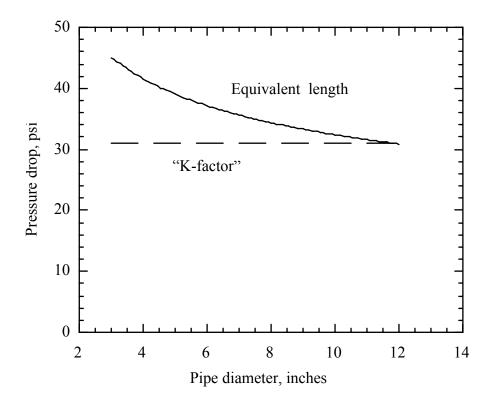
We see that the equivalent length estimate is higher than the "K-factor" estimate for small pipes, but that the two values cross at about 1 ft. I ran the value for 24 inches on the same spreadsheet program, finding  $dP \approx 6.5$  psi. I don't know which is best, other than to follow Lapple's suggestion in the text.
