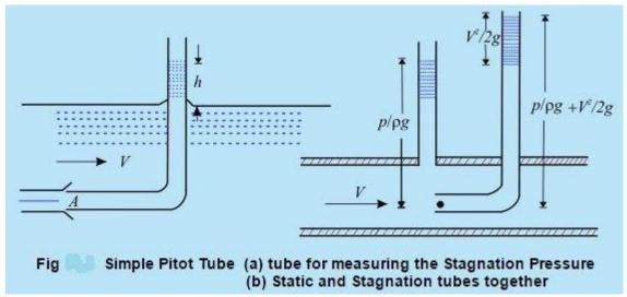
A pitot tube is an open-ended right-angled tube pointing in opposition to the flow of a fluid and used to measure pressure.
