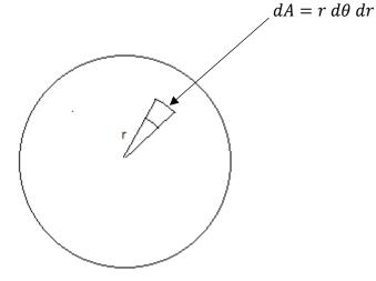
V is the local velocity measured by a Pitot tube at a distance r from the center of the tube. It is function of r only and independent of  $\theta$  due to symmetry.
