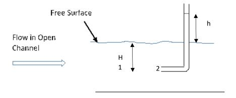
Some of the liquid enters the tube and rises in it to a height h above the free surface of the liquid. This is equivalent to converting kinetic energy into potential energy. The velocity at a point below the surface at a distance H (point 1) can be found by applying BE between points 1 and 2. Point 1 is considered far from point 2 so that it is not affected by the presence of the tube. Point 2 is just at the entrance of the tube.
