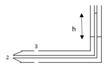
The inner tube faces the flow point 2; while the outer tube has holes tangent to the flow point 3. The inner tube measures the total head (static + dynamic); while the outer tube measures the static head or Piezometric head (points P1 or P2).
