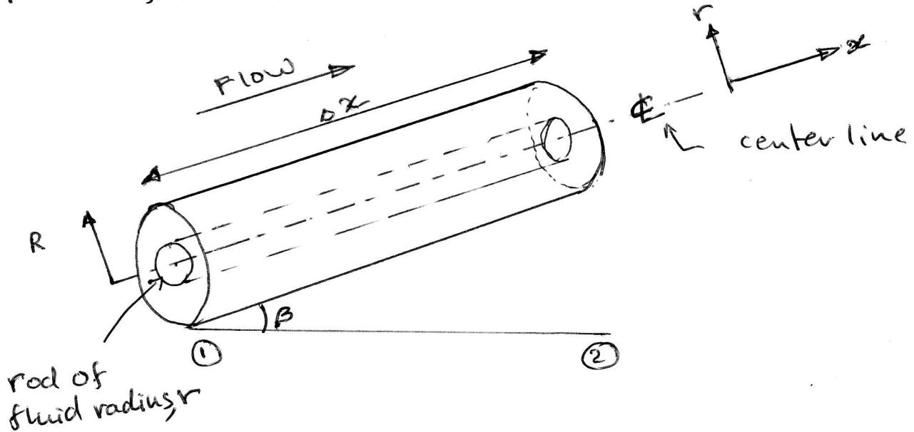
Make a force balance on a rod of radius( $r$ ) under the following conditions:
