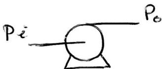
A pump adds energy to a flowing fluid. This energy raise the pressure from  $P_i \rightarrow P_o$  ( $P_o > P_i$ )
