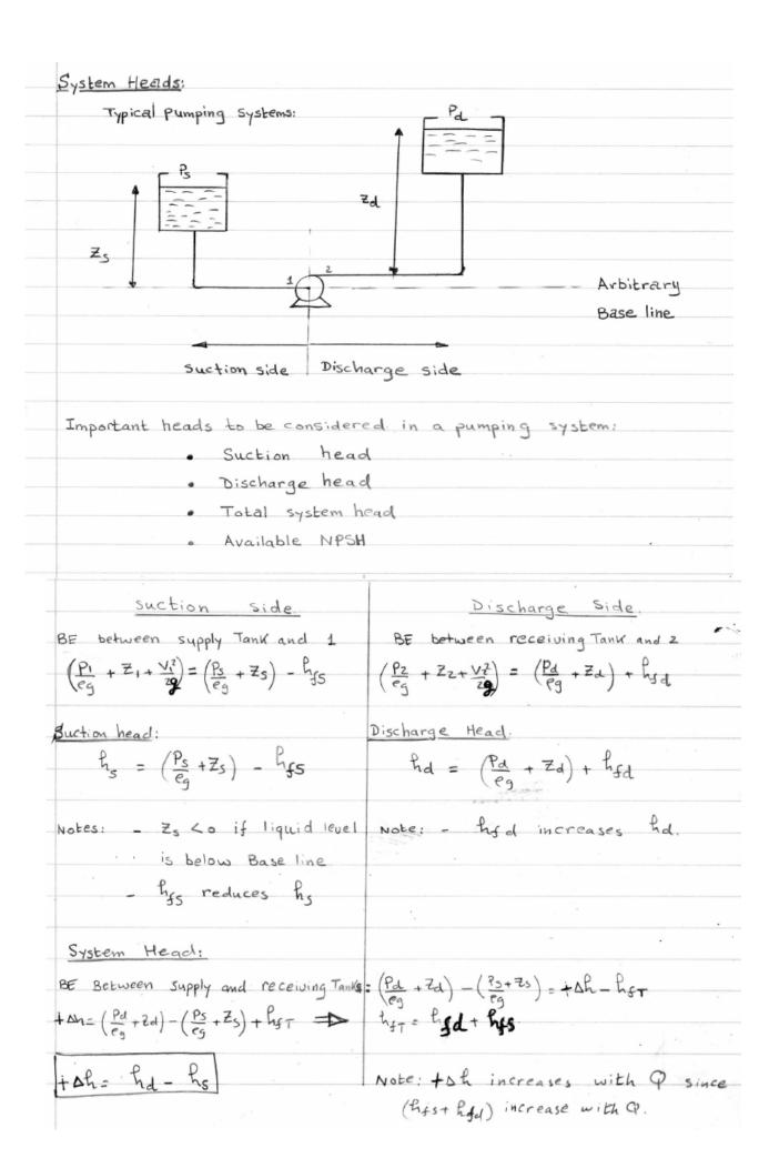
This is the total head which should be imparted by the pump to the fluid for a certain flow rate. It is called the **System Head**. It is the work required to be done by the pump for a certain system at a certain flow rate.
