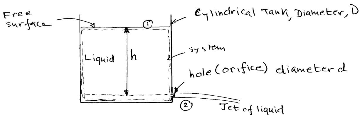
Definition of system: Liquid as indicated between level ① free surface (considered as input to system) and plane ② just outside the tank (considered as output from system).
