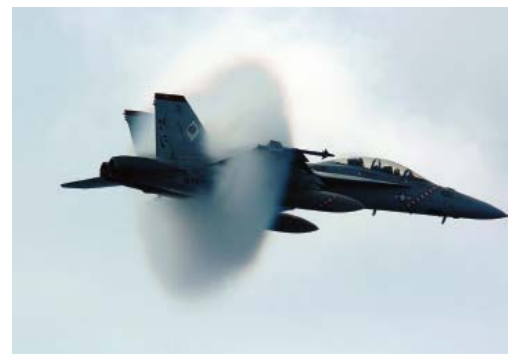
The sudden drop in temperature produces condensation of water vapor on a visible vapor cloud when an aircraft flies near the speed of sound.
