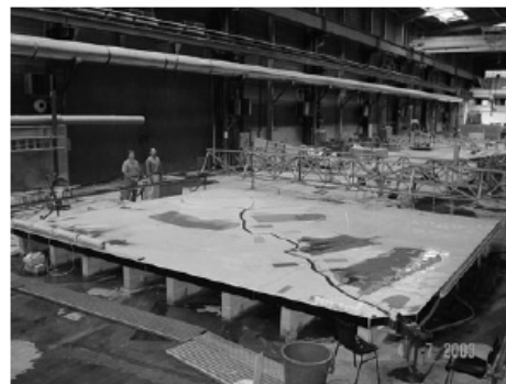
scale model of a section of the Mississippi River.
