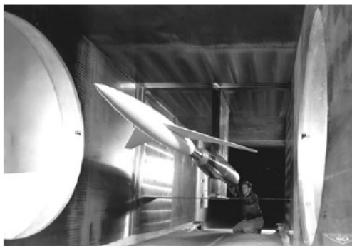
Model of an aircraft in a wind tunnel.
