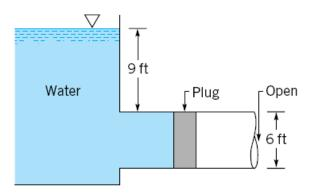
**Problem 7.** A tanker truck carries water, and the cross section of the truck's tank is shown in figure below. Determine the magnitude of the force of the water against the vertical front end of the tank.
