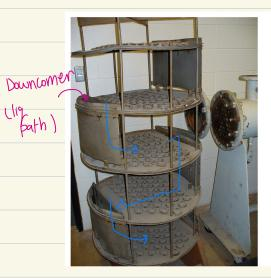
\* lig level has a pressure head that is sufficient enough that it won't carry over by the vapor
