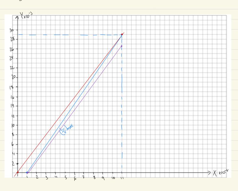
$$\frac{L}{V} = 0.9 \left(\frac{L}{V}\right)_{\text{max}} = \frac{28.9 \times 10^{-3} - 0}{11 \times 10^{-4} - 1 \times 10^{-4}} = 28.9$$
