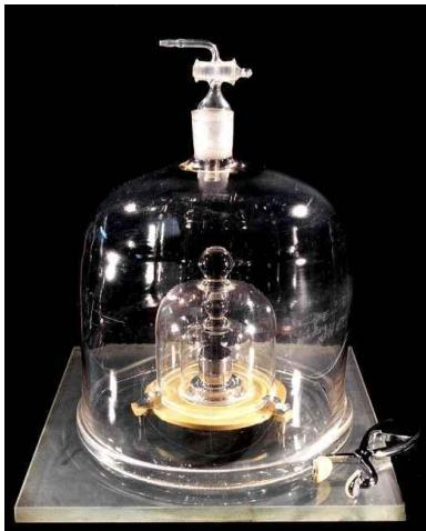
Fig. 1. The official kilogram reference cylinder (left) and its copy (right) at the International Bureau of Weights and Measures in Sevres, France.
